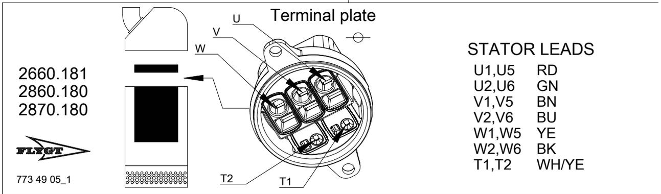
STATOR LEADS AND THERMAL CONTACTS
